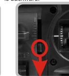
油门微调: 注意在飞行时或在调机子时, 油门微调一定要打与最底。 Throttle trimmer: Note that the throttle trimmer must be pushed down to the lowest when flying or adjusting the plane.
