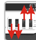
伺服器倒置开关: 出厂前倒置开关已调好, 没有必要时无须再调。右手开关: 下上上上左手开关: 下上上上。 switch has been adjusted in the factory; it does not need to be adjusted any more if there is no necessary.
