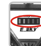
LED 指示灯: 灯全亮时说明电池电量最多, 只亮最后一个红灯时说明电量快用净, 需马上更换。 LED indicating light: when all the lights are on, it indicates that the quantity of electric charge is fullest; when only one red light is on, it indicates that the battery almost used up and it need change immediately.
