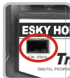
晶体接插孔: 在装晶体时要特别小心, 因接插孔比较深。 Crystal plug board hole: please watch out when assembling the crystal because the hole is comparatively deep.
