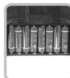
电池盒: 注意正负级别, 切勿装反。 The battery box: notice its positive and negative. Never assemble it in the reverse direction.
