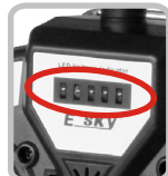
LED 指示灯: 灯全亮时说明电池电量最多, 只亮最后一个红灯时说明电量快用尽, 需马上更换。 LED indicating light: when all the lights are on, it indicates that the quantity of electric charge is fullest, when only one red light is on, it indicates that the battery almost used up and it needs change immediately.
