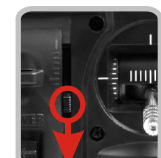
油门微调: 注意在飞行或调试时, 油门微调一定要打与最低。 Throttle trim: Note that the throttle trim must be pushed down to the lowest when flying or adjusting the plane.
